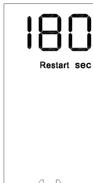
Compressor Protection Status
