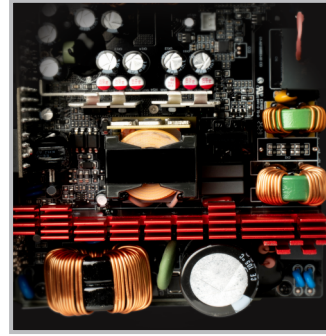
Full-Bridge Resonant, High-Efficiency 12V-Centric Power Design
