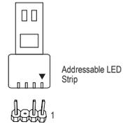
Connect your addressable LED strip to the header. The power pin (marked with a triangle on the plug) of the LED strip must be connected to Pin 1 of the addressable LED strip header. Incorrect connection may lead to the damage of the LED strip.
