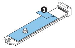
If you want to install 22110 SSD, use the included EZ M.2 Clip II Remover to remove the EZ M.2 Clip II in the 2280 hole. And then secure the included M.2 plate screw in the 2280 hole. Skip this step if you install 2280 SSD.
