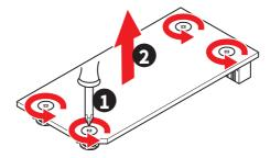
3. If you install 2260 SSD, use the included **EZ M.2 Clip II Remover**. Place the included **EZ M.2 Clip II** in the slot, use the remover to screw it in by turning clockwise, and secure it. Skip this step if you install 2280 SSD.
