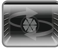
**Fan Function:** The oven's thermostat and warning lights will switch on, and the upper and lower heating elements and fan will start operating.
