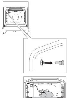
Remove the metal cap (the socket is located in the front upper corner of the oven right wall).
