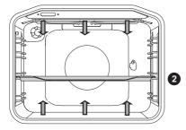
The heaters in the bottom and in the ceiling of the oven cavity will radiate heat evenly into the oven interior.
