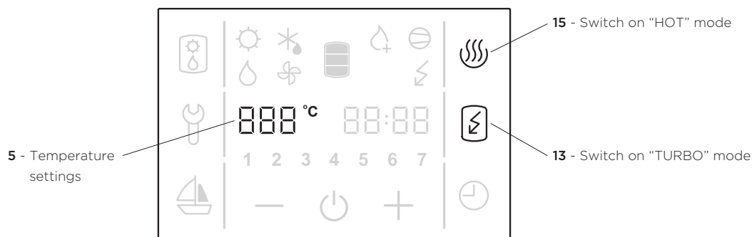
Figure 11: Temperature settings, switch on "TURBO" and "HOT" mode
