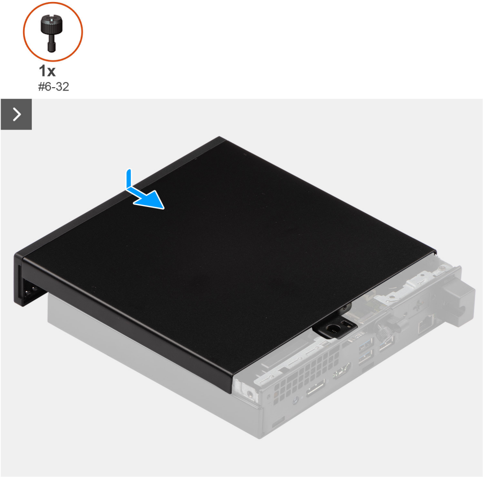
Figure 11. Installing the side cover
