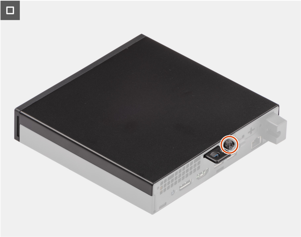
Figure 12. Installing the side cover
