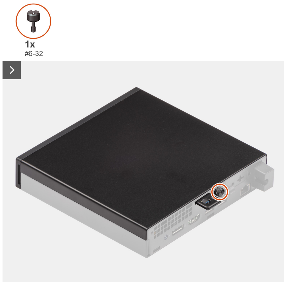
Figure 9. Removing the side cover
