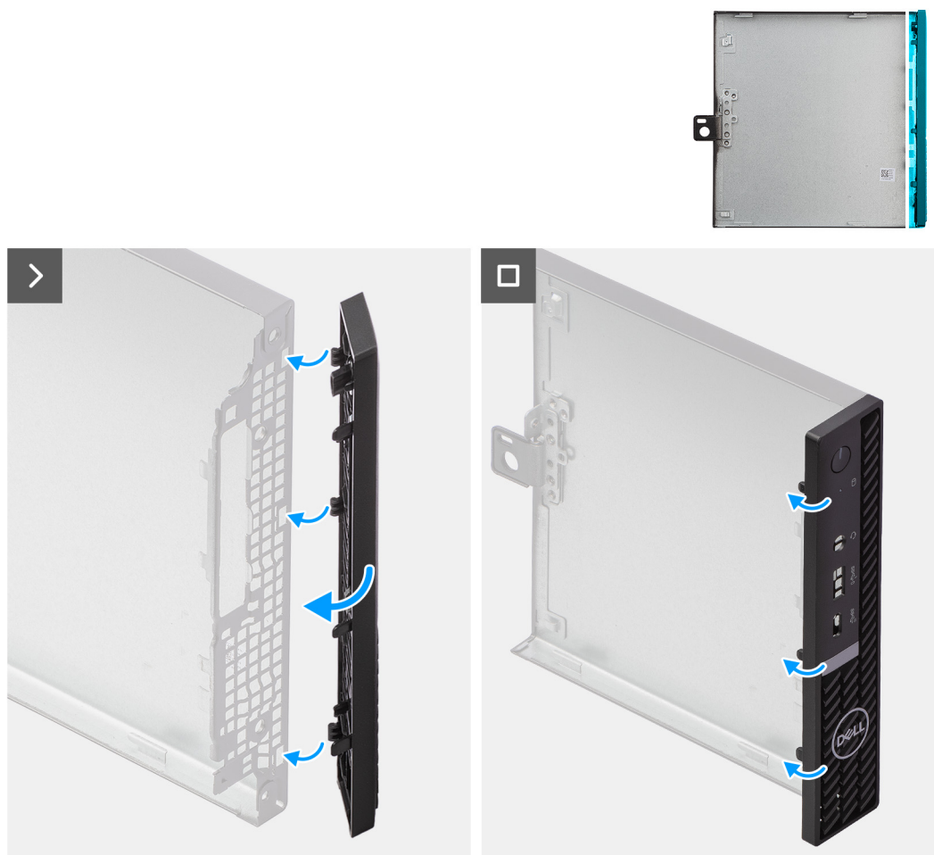
Figure 16. Installing the front bezel
