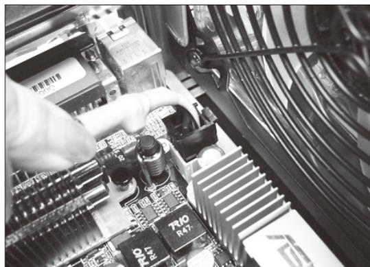
▶ Connect the 4+4 pin auxiliary power connector to the motherboard.
