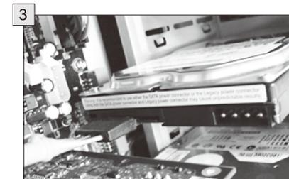
▶ If you have S-ATA disk drives, connect the Serial ATA connectors provided.
