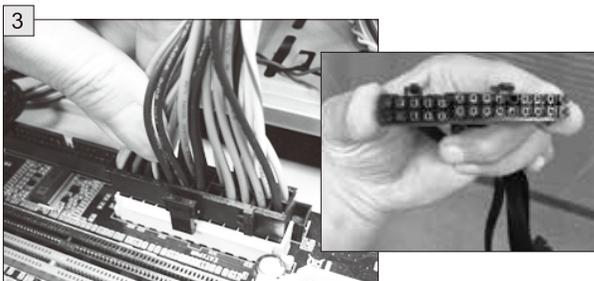
▶ After installing the power supply unit into the chassis, connect the 18+10-pin main power cable to the 20 pin or 24 pin motherboard socket.
