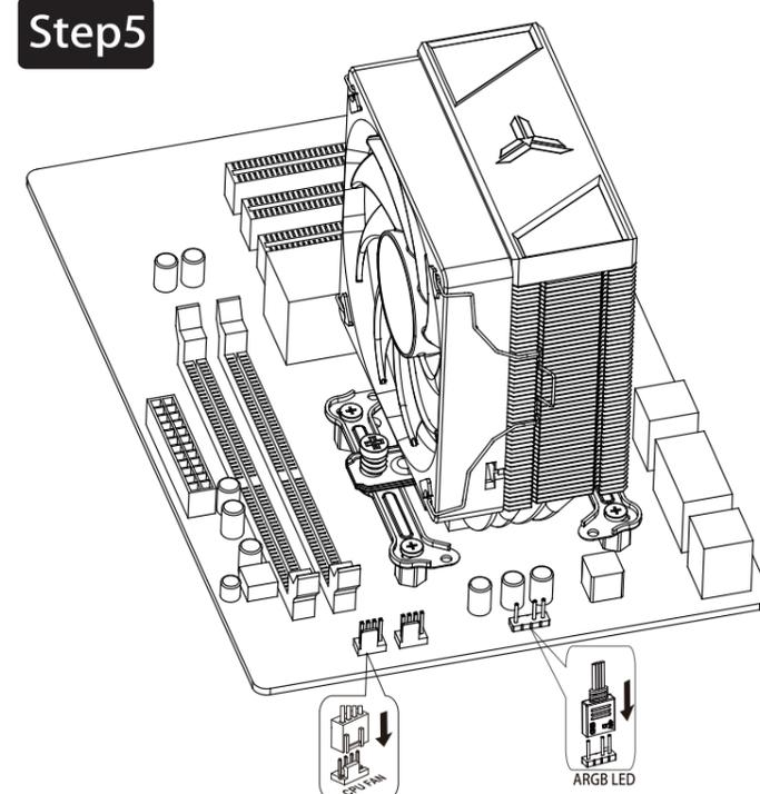
Connect the fan lead to the main board as shown in the figure above
