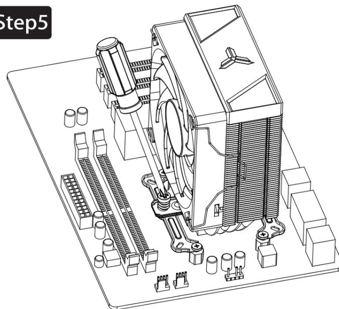
Place the cooler on the CPU while aligning the screws to the backplate mounting points, secure with screwdriver.
