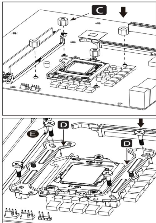
Install the mounting brackets and secure with screw
