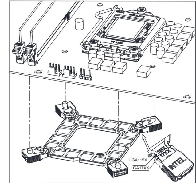
Install the backplate to the motherboard and fix it with spacers
