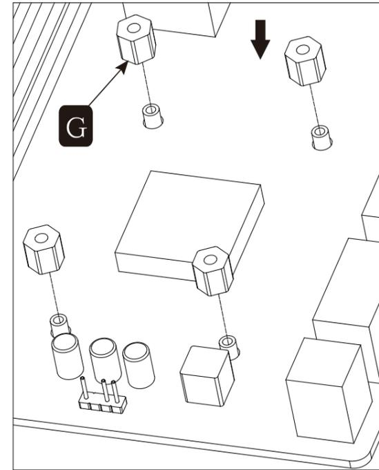
Installation of AMD spacer column
