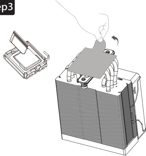
Applying the thermal paste on CPU evenly, and remove the protection film from copper base
