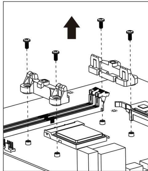
Remove the plastic retainer of the AMD retention module, place the existing backplate back to MB
