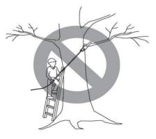
Never work from a ladder or other unstable equipment while working with a chain saw. Always grasp the chain saw with both hands. While cutting, apply firm and continuous pressure on the chain saw but do not try to force the chain saw through the wood being cut. Do not use the chain saw for cutting branches having larger diameter than the length of the guide bar.
