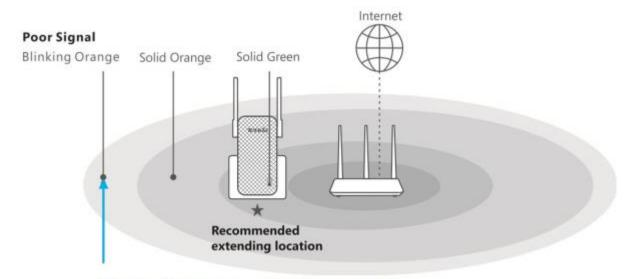
If the signal is very poor, you must keep moving the extender to an outlet closer to the router until the LED indicator of the extender lights solid green or solid orange.
