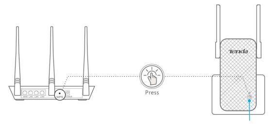
When the LED indicator turns to solid green, solid orange or blinking orange, it indicates that the WPS connection is successful.
