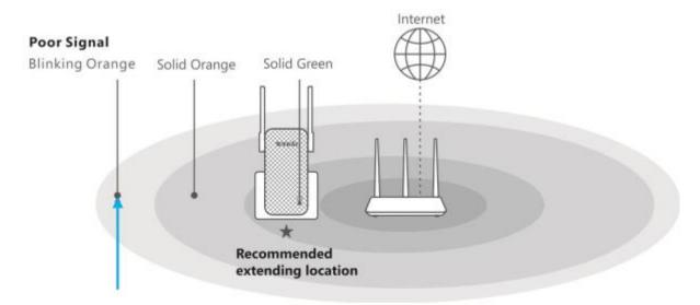
If the signal is very poor, you must keep moving the extender to an outlet closer to the router until the LED indicator of the extender lights solid green or solid orange.
