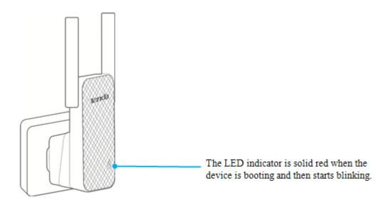
② Use your computer to search and connect to the extender's WiFi. The default WiFi name (SSID: Tenda\_XXXXXX) is on both the label of the extender's rear panel and the label of the extender's side panel, shown as below.
