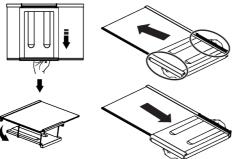
To group the wine rack, first remove the glass shelf from the refrigerator. Place it on the glass shelf by pushing the plastic part through the front and back grooves as shown in the picture. The product will be ready to use with the foldable wine rack. To remove the foldable wine rack, first remove the glass shelf from the refrigerator. Then grab the plastic part and pull it in any direction. You can now use the product without a foldable wine rack when needed.
