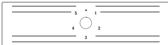
Freezer thermostat automatically regulates the inside temperature of the compartments. By rotating the knob from position "1" to "5", colder temperatures can be obtained.
