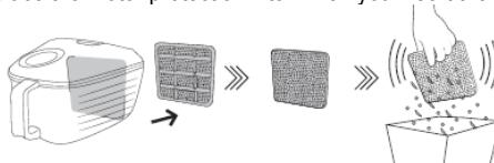
Remove the holder. // Insert the bottom edge of the new filter properly into the ridges of the holder. // Close the holder by pressing it back into place gently. Make sure that the filter fits completely into the holder.
