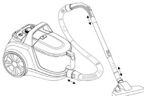
To connect the suction hose: insert the suction hose into the opening.
