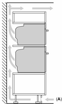
A: Dovod vazduha  $\geq 200 \text{ cm}^2$
