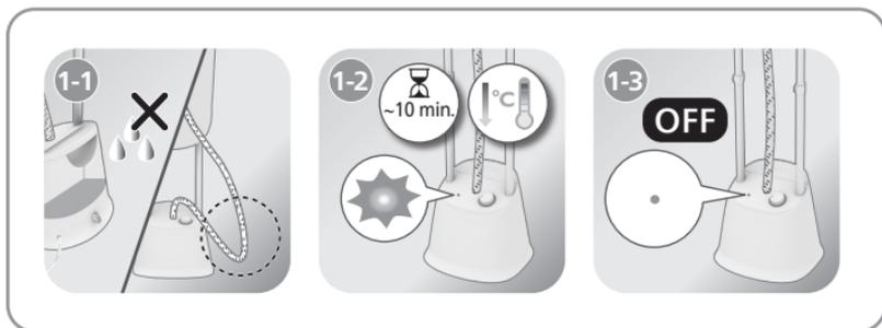
**EN** **Figure 1-1:** The appliance will go into auto-off mode (LED light will blink) when the water tank is empty or when the steam hose is bent.
