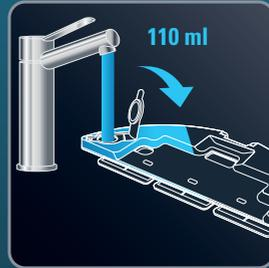
**EN** Open the water tank of the mop support and fill it with 110ml of water.
