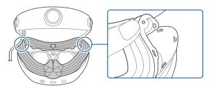
Be careful when removing or attaching the light shield, as it may break if you use excessive force.
