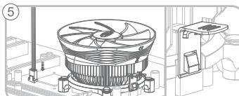
Press down the other side clip and hook it onto the tab, too. And then finish the installation by connecting the fan cable to the motherboard.
