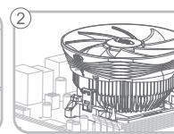
As illustrated, put the heatsink onto the processor and hook the vertical dip onto the retention frame tab.
