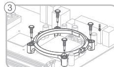
As illustrated, put the heatsink onto the processor and hook the vertical clip onto the retention frame tab.
