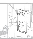
Press down the other side clip and hook it onto the tab, too. And then finish the installation by connecting the fan cable to the motherboard.
