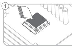
Evenly apply a thin layer of thermal grease onto the processor.
