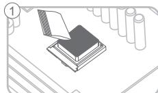
Evenly apply a thin layer of thermal grease onto the processor.
