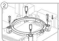
Attach the mounting bracket onto motherboard by inserting the clips into the right holes according to socket type.
