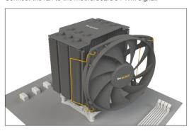
When dismantling the 135mm fan, push the notches of the fan clips away from the fan.
