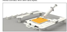
Position the cooler mounting bridge centrally on the cooler. Next place the cooler unit onto the CPU. Insert the mounting bridge fastening screws from above into the cooler mounting bridge and then screw these alternately tight.
