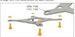
For fixing the backplate screws onto the Intel backplate use the O-rings. Once assembly of the Intel backplate for the respective Intel socket is complete, position it under the motherboard. Make sure that the backplate screws are precisely positioned inside the motherboard holes.
