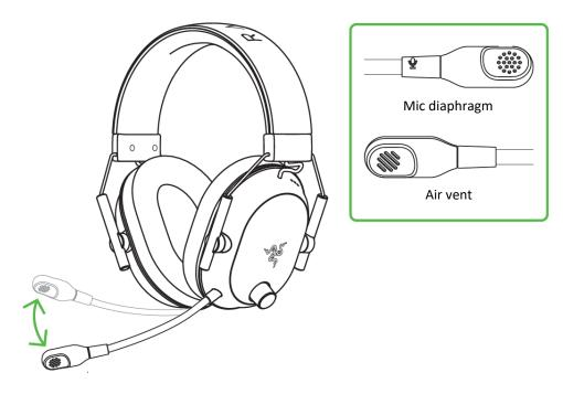
The recommended mic-to-mouth distance for optimal sound capture is 1.5 cm to 3 cm (0.59 in to 1.18 in).
