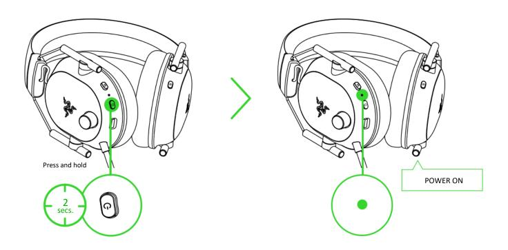
3. Wait for the headset indicator LED to turn solid green, indicating that the headset is now connected to the wireless dongle.
