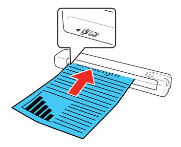
• For longer originals, slide your original into the input slot against the left side as shown until it meets resistance. Make sure the printed side is faceup and top edge first. Set the paper size in the scanning program and support the original as it enters into and ejects from the scanner.
