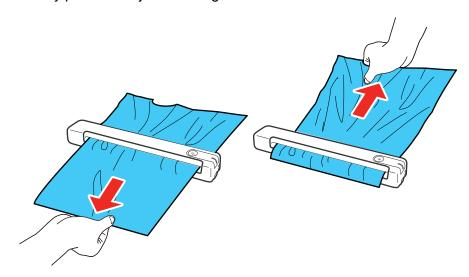
**Note:** Pull the jammed original gently, otherwise it could be damaged. If paper gets stuck in the roller and remains inside the scanner, carefully remove it with a pair of tweezers in the direction of the output slot. If you cannot remove it, contact Epson for support.
