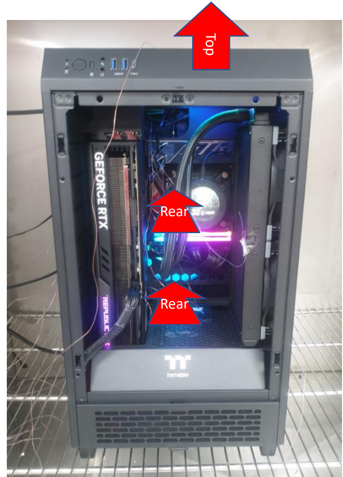
Hot Airflow Exhausts
