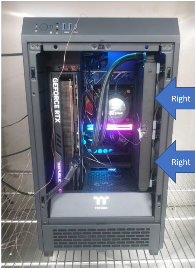
Cool Airflow Inlets (Active)
