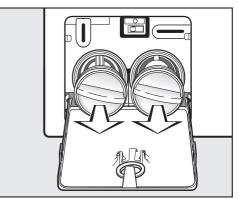
Remove the drain filters completely.
