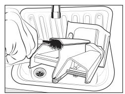
Clean the fabric conditioner channel using a brush and warm water.
