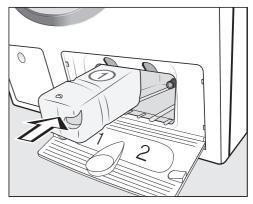
Push the UltraPhase 1 detergent cartridge into compartment 1 until it locks into position.
