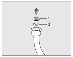
Remove the rubber seal 1 from the recess.
