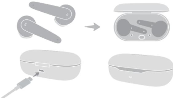
**EN** Earphones: Place the earphones in the case and the earphones automatically start charging.
