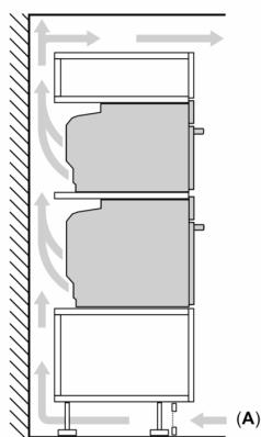
A: Dovod vazduha  $\geq 200 \text{ cm}^2$
