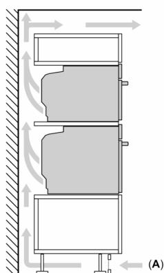
A: Dovod vazduha  $\geq 200 \text{ cm}^2$
