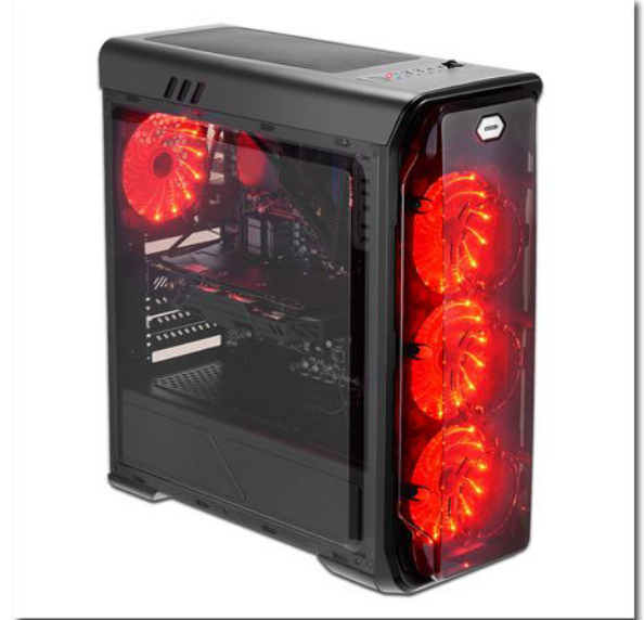
- incl. four red lighted 120 mm LED case fans
