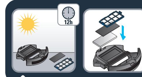
**EN** Let all parts dry approximately 12 hours. Do not use wet filter or dust container. When dry put the filters back in the dust container.
