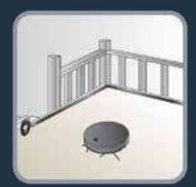
**EN** The robot has drop sensors to detect stairs and gaps. The robot will change direction when detecting them. In order to correctly detect the floor level difference, make sure there are no objects (bags, shoes...) on the floor next to gaps, stairs or on the stairs' steps. The step must be more than 10 cm away to be detected. If the area to be cleaned has stairs, a magnetic strip must be placed at the edge of a drop in order to prevent product damage and ensure safe operation.
