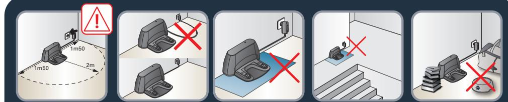
**EN** To place the docking station, make sure there is an empty area of 1.5m on each side and 2m in front of the docking station. Do not install the docking station near stairs. The cable must be tight. Always place the docking station on hard floor. Do not place the docking station on carpet.
