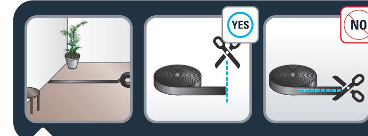
**EN** Should you like to restrict access of the robot to some areas, use the magnetic stripe. Put the magnetic stripe on the floor to mark a no-go zone for the robot.
