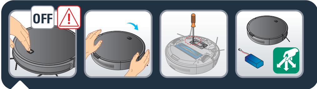
**EN** Attention: Before removing the battery turn off the robot. Turn the robot upside down to get access to the battery slot. Remove the battery by screwing the topcover. Disconnect the battery from the robot. Recycle the battery and robot.
