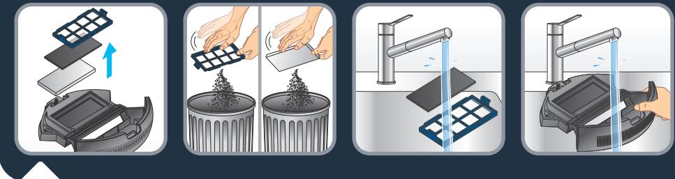
**EN** Clean the filter cover and the filter by tapping the back, holding it above a waste bin. Wash the foam filter, the filter cover and the dust catcher in clean water. Do not wet the fine dust filter (white filter). The filters must be cleaned at least once a week.
