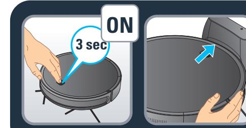
**EN** To charge the robot turn it on by pushing the on / off button for 3 seconds. Place the robot on the docking station: the charging plates on the robot must touch those on the docking station. Replace the robot on its charging base after use.
