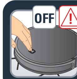
**EN** Attention: Before touching sensitive parts of the robot make sure it is turned off by pressing the on / off button 3 seconds.
