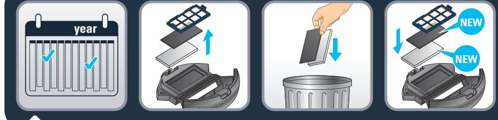
**EN** Every 6 months replace the fine dust and foam filter with new ones to maintain optimal performance.
