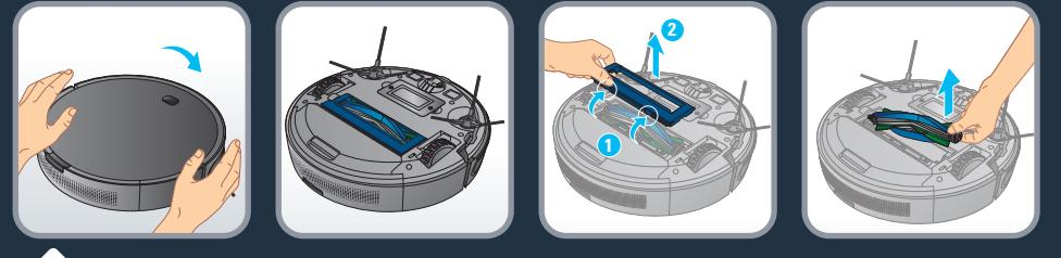
**EN** Clean the brush of the robot once a week. To do that turn the robot upside down. To remove the brush, open the brush guard by pushing the 2 snap latches and pull it up. Then pull out the brush from the robot.
