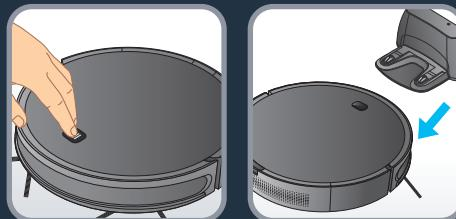
**EN** To clean all the accessible areas of your home, use the « Methodic » mode: press once the Power button. To clean a localized area of your home, use the « Spot » mode: press twice the Power button. Please note that the « Spot » mode is not available when the robot is on the docking station. To clean along the walls and in the corners, use the « Wall follow » mode: press three times the Power button.
