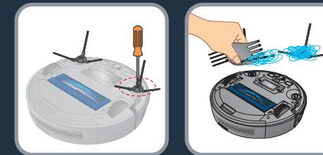
**EN** To clean the side brush, remove it and use a cleaning brush to clean the side brush and the entanglements in the slot of the side brush. Replace lateral brushes every 6 months.
