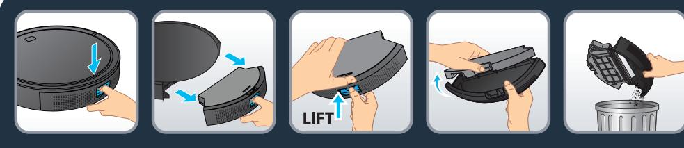
**EN** The robot must be emptied and cleaned after each use. Push the button on the backside of the robot and pull out the dust container. To empty it, flip off the cover.
