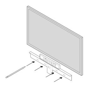
Use a 5/16" drill bit to drill pilot holes.
