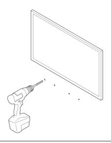
Insert and secure the wall anchors (don't use the anchors if drilling into wood).
