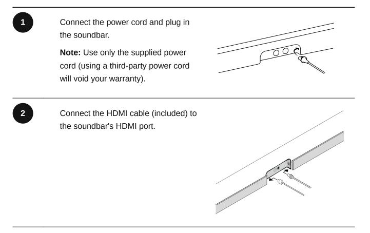
If your TV has an HDMI ARC (or eARC) port, connect the HDMI cable to it.
