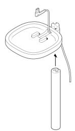
Use the 2 silver screws to attach the speaker platform to the top of the stem, threading the power cable carefully. Snap the bottom plate on with the power cable channel in the back, and mount the platform on the stem.
