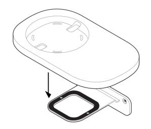
Position the Shelf the way you want it (supports left or right speaker placement). Press the Shelf firmly on to the wall bracket until it snaps into place (both front and back).
