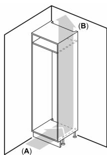
A: Air inlet  $\geq 200 \text{ cm}^2$ ; Ventilation options
