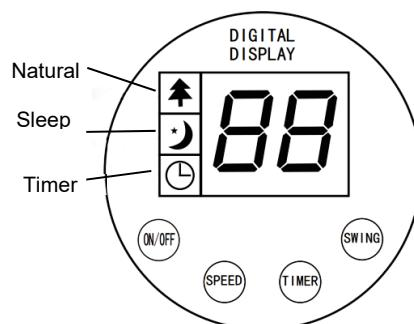
**Note:** The remote control has the same functions as the control panel, except for the MODE function which is only possible via the remote control.
