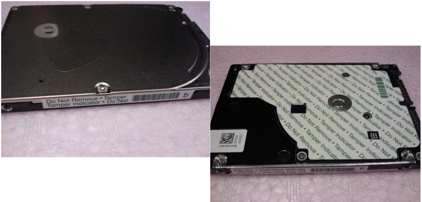
Figure 9 Example of FIPS tamper evidence labels.
