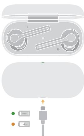
**EN** Place the earbuds in the charging case to initiate automatic charging. Use a USB-C cable to charge the charging case.
