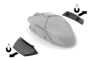
2. Magnetically connect the thumb rest blank.
