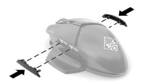
▲ To replace a set of programmable buttons, reverse this procedure.
