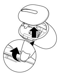
2 Remove the USB dongle from its compartment.
