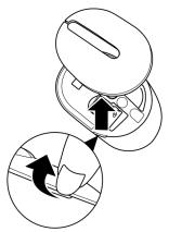
2 Remove the USB dongle from its compartment.
