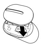
5 Slide the power switch to turn on the mouse.
