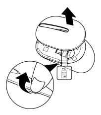
2 Remove the USB dongle from its compartment.
