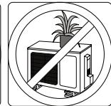
Make sure nothing is blocking all air inlets and outlets
