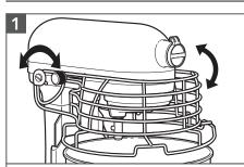
To attach the Bowl Guard\*: Make sure that the guard is returned to the down position before beginning to use the Stand Mixer. The Stand Mixer will not run if the Bowl Guard is not in the proper position.
