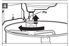
To attach the accessory: Slip the accessory onto the shaft. Turn to hook it over the pin on the shaft.
