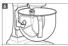
Test the beater to bowl clearance: Plug the Stand Mixer into an earthed outlet. Turn Stand Mixer ON and test each speed, making sure the beater does not touch the bowl during operation. If the beater is too far away from the bottom or is hitting the Bowl, proceed to next step to make adjustments.
