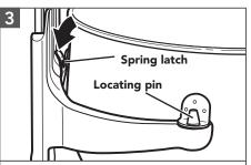
To attach the Bowl: Fit the Bowl Supports over Locating Pins and press down on back of the Bowl until Bowl Pin snaps into spring latch.
