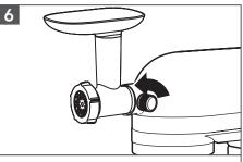
Loosen Attachment Knob by turning it counterclockwise. Rotate attachment slightly back and forth while pulling it out.
