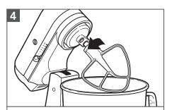
**To remove accessory:** Repeat steps 1 and 2. Press accessory upward as far as possible and turn to the left. Then pull accessory from the Beater Shaft.
