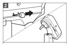
Unlock and lift the Motor Head. The lock\*\* engages automatically to keep the head locked in place.
