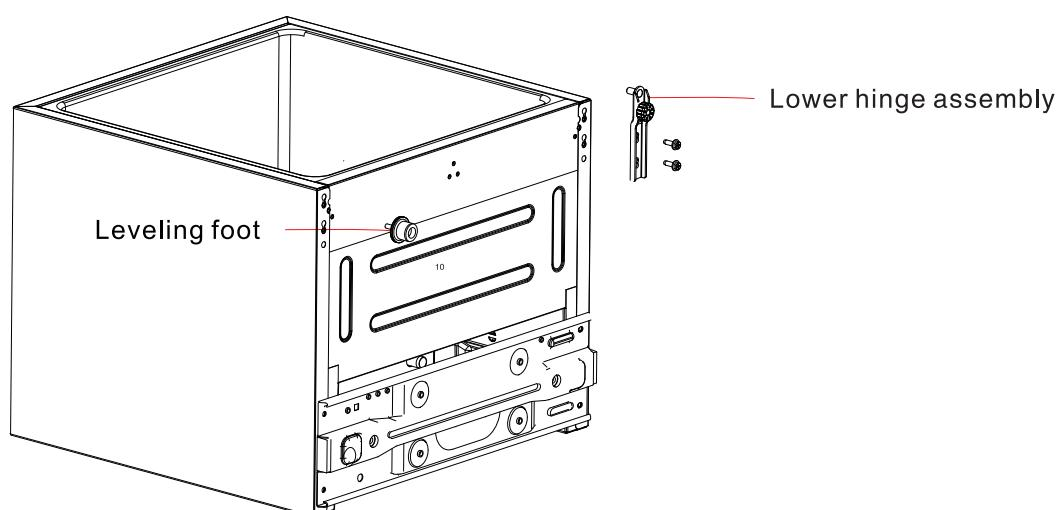
5) Install the lower hinge and leveling foot on lower left side of cabinet and lower right side respectively;
