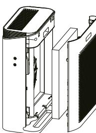
Place the filter back into the purifier with its little handle facing outwards.
