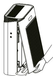
Replace the filter cover and connect to the power source.
