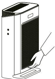
Remove the filter cover by pulling the bottom handle
