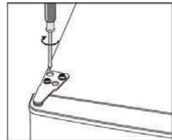
10. Put the hinge cover and the screw cover back.
