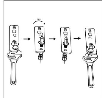
6. Refit the bracket fitting the bottom hinge pin. Replace both adjustable feet.
