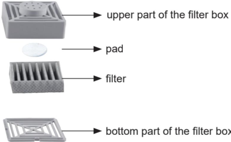
Close the filter box and replace it into the appliance. Close the appliance by fixing the bottom cover to the main body by rotating it clockwise.
