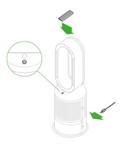
Place the remote control on top of the machine with the buttons facing down.
